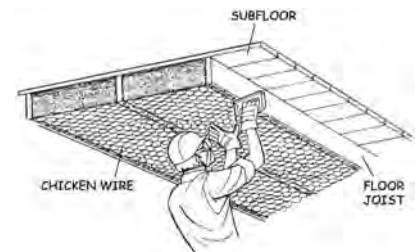
FIG. 39-6: INSTALLATION OF WOVEN WIRE
