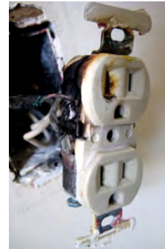
FIG. G-3: RECEPTACLE WITH CHARRING
