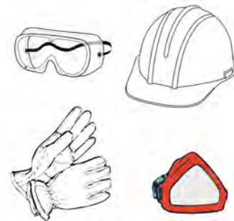
FIG. G-2: PERSONAL PROTECTIVE EQUIPMENT
