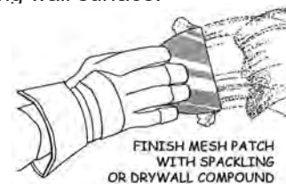
FIG. 32-18: MESH PATCHES ON FLOORS
