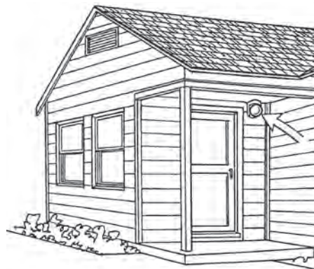
FIG. 28-1: EXAMPLE OF A DAMP LOCATION
