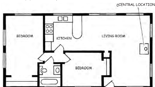
FIG. 4-27: WOOD STOVE/INSERT CENTRAL LOCATION
