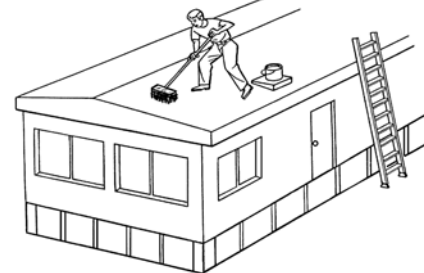
FIG. 37-7: ROOF LEAKS MUST BE REPAIRED BEFORE INSULATION IS INSTALLED
