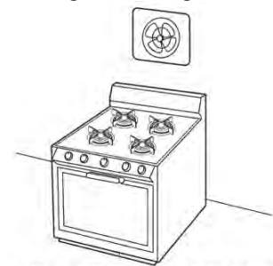
FUNCTIONAL VENTILATION REQUIRED IN COOKING AREA OF A MOBILE HOME FIG. 21-5: FAN OR PASSIVE VENT REQUIRED IN MOBILE HOME COOKING AREA
