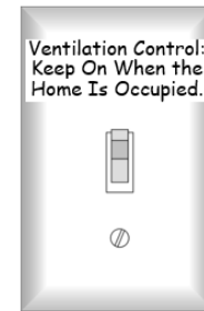
FIG. 12-8: LABELED SWITCH FOR MECHANICAL VENTILATION OVERRIDE CONTROL
