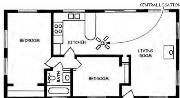
FIG. 24-1: CORRECT FAN LOCATIONS
