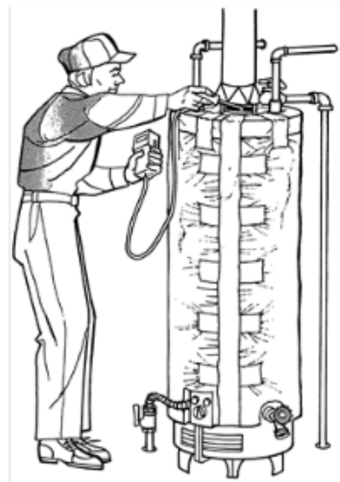
TEST PROBE/EXTENSION IS PLACED INSIDE THE CENTER TUBE ON EACH SIDE OF THE BAFFLE
