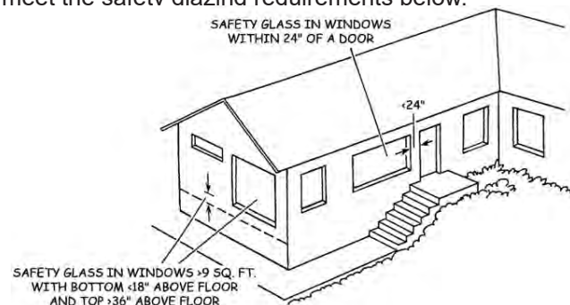
FIG. 2-11: REQUIRED LOCATIONS FOR SAFETY GLASS
